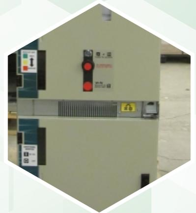
**Lockable access to the VCB racking in/out mechanism** by a metallic shutter prevents unauthorized operations and interlocks the VCB in the trip position prior to racking a draw-out unit.
